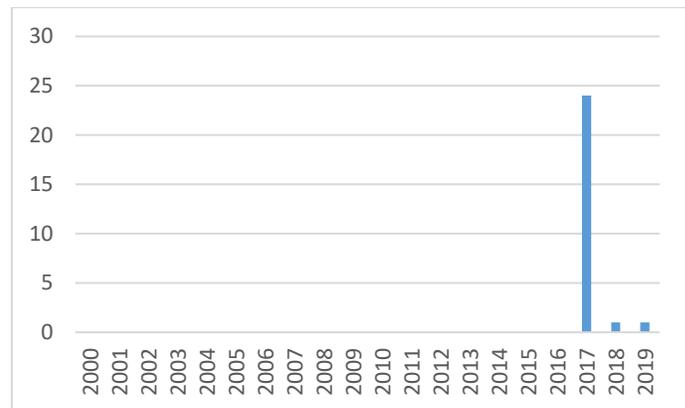
**FIGURE 12:** ANNUAL NUMBER OF CRACKS FOR FPSO 6. THIS FPSO HAS BEEN IN SERVICE SINCE 2011.
