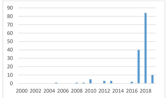
**FIGURE 10:** ANNUAL NUMBER OF CRACKS\*) FOR FPSO 4. THIS FPSO HAS BEEN IN SERVICE SINCE 1999.
