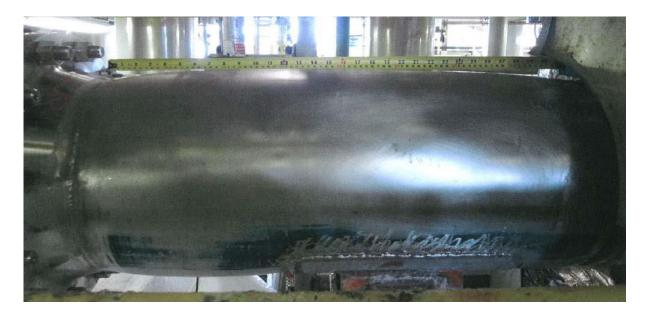
Figure 11: Deformed pipe section between HCV 20021 and the leak site. (Source: Statoil's investigation report)
