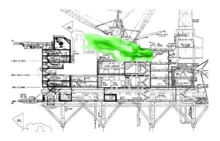
Figure 9: Facade drawing with a projected gas cloud, viewed from south to north. (Source: Statoil's Flacs analysis)
