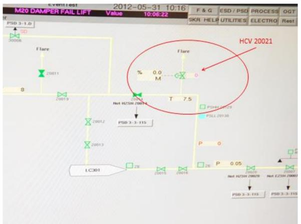
Figure 6: The CCR operator had a limited overview of the valve configuration.
