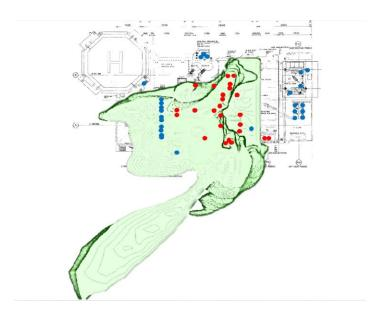
Figure 10: Gas cloud projected down to the weather deck at 230 seconds into the incident. Red dots show detectors, which activated at 20 per cent LEL. Blue dots show detectors which did not detect gas during the incident. (Source: Statoil's Flacs analysis)
