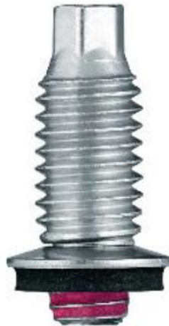
Figure 24: S-BT GR Threaded screw-in stud (stainless steel, metric thread) for grating fastenings on steel and aluminium in highly corrosive environments.
