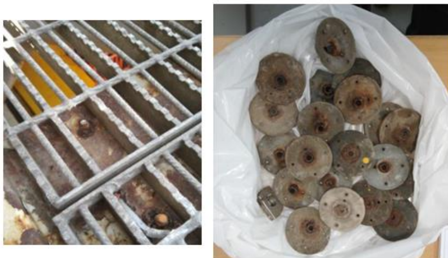
Figure 18: Galvanic corrosion of fasteners.
