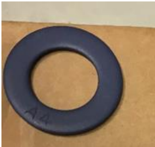
Figure 27: 316 SS washer with 10 – 15 \mu\text{m} , PTFE, type Xylan 1070 Blue.
