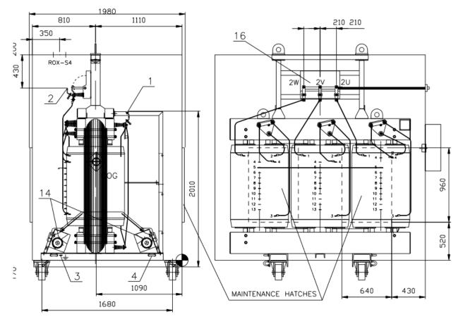
\*) Minimi clearance to deck if the rollers are removed. Figure 11: Arrangement drawing of the transformer. Source: Equinor
