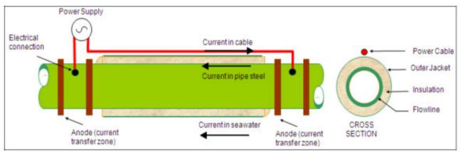
Figure 8: Direct electric heating (DEH) system – open loop (wet insulated)
