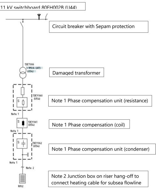
Figure 9: Extract from single-line diagram for the DEH system.
