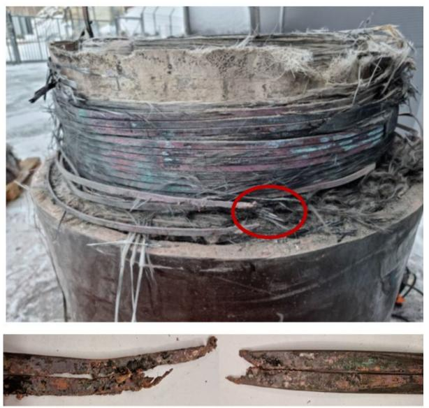
Figure 14: Defective/melted copper winding on the secondary side located at the top of the middle coil.
