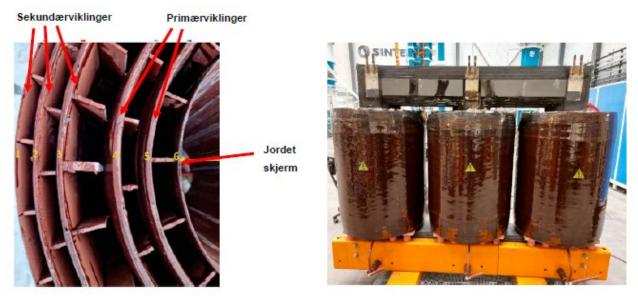
*Figure 12: Images of the transformer with windings and core. Source: Sintef* Key: Secondary windings Primary windings Earthing screen
