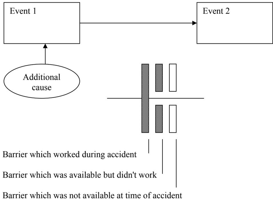
Figure 1: Sample barrier diagram.
